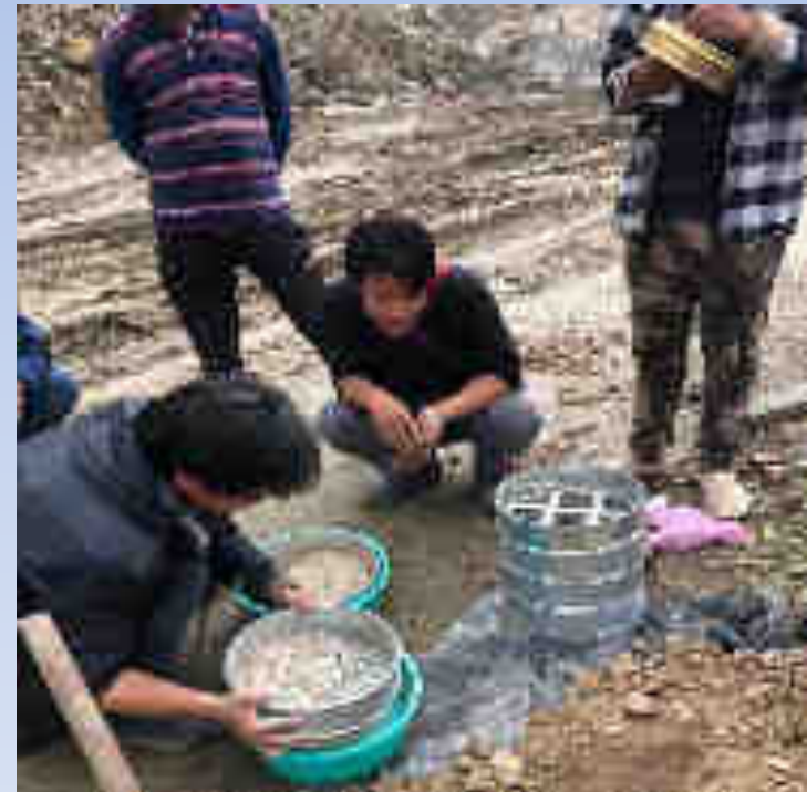
Gradation Test at Site
